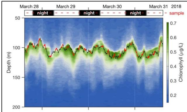
Figure 5: Time-series measurements of chlorophyll profiles during an ESP/LRAUV drift. The solid black line represents drift depth, as controlled by AUV autonomous isotherm tracking. ESP sampling events are shown by the red line segments. Times of discrete measurements conducted by shipboard CTD sampling for comparative purposes are shown by solid black circles.
